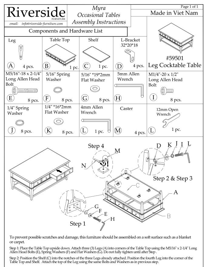
Step 3: Attach the Shelf to the Legs using the L-Brackets (D) and the  $M1/4" \times 1/2"$  Long Bolts (I), Spring Washers (J) and Flat Washers (K). While pulling the Legs into the notch, tighten the Bolts with the Allen Wrench (L). Fully tighten all the bolts with Allen Wrench (H).
