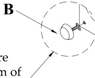
Adjustable levelers are installed in the bottom of the Legs and can be adjusted to compensate for uneven flooring if needed.
