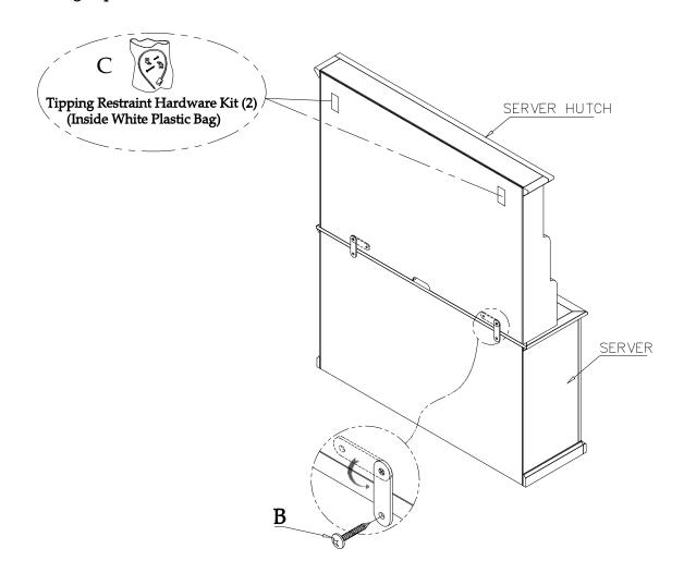
Step 1: After the Server has been moved to near its final location in the room, position and connect the Server Hutch on top of the Server. Pivot the Mending Plates attached to the back of the Hutch down and using your Phillips Screwdriver install the Wood Screw (B) to connect the pieces together.
